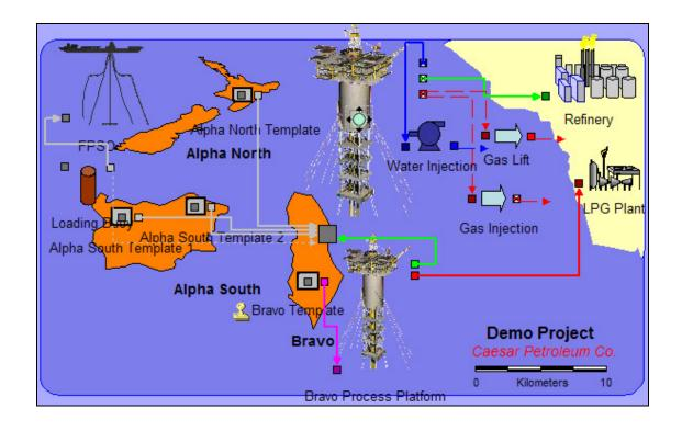
PetroVR Surface Layout is the place where facilities and pipelines are built and connected, defining a fluid routing strategy -a crucial part of the simulation.
